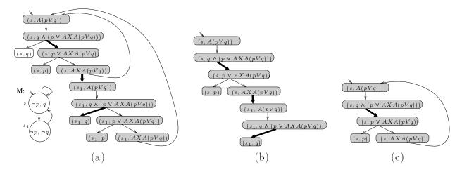
Figure 3.1: (a) A colored game-graph for M and  $\varphi = A(pVq)$ , where white nodes are colored by T, grey nodes are colored by F and bold edges point to the *cause* of an  $\wedge$ -node, (b) Its annotated counterexample computed by ComputeCounter, and (c) A possible result of ComputeCounter without the use of the *cause* in  $\wedge$ -nodes.
