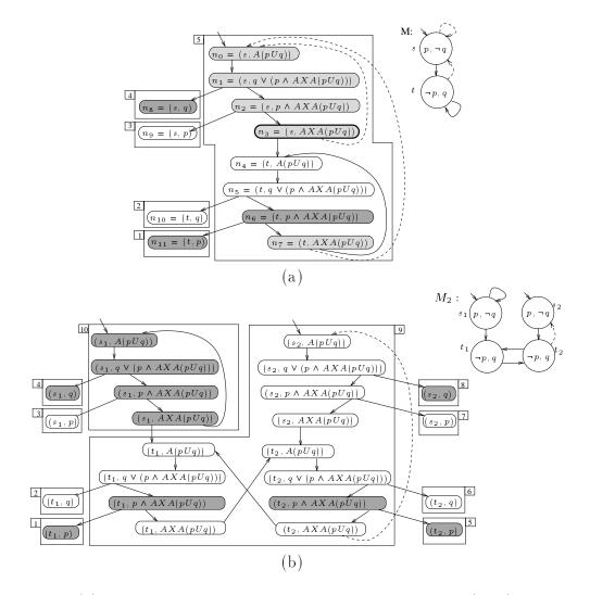
Figure 6.1: (a) A 3-valued colored game-graph for M and  $\varphi = A(pUq)$ , where the initial node is colored by ? and the failure node found by FailureSearch appears in boldface; (b) The colored refined game-graph, based on the refined model  $M_2$  and  $\varphi$ .
