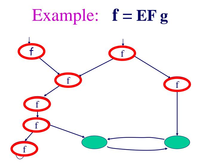
Model checking  $\mathbf{f} = \mathbf{E}\mathbf{G}\mathbf{g}$ **CheckEG** gets  $M = \langle S, I, R, L \rangle$  and  $S_{g}$ and returns  $S_{f}$ procedure CheckEG  $(S_{\sigma})$  $\mathbf{Q} := \mathbf{S}; \mathbf{Q}' := \mathbf{S}_{g};$ while  $Q \neq Q'$  do **O** := **O**';  $\mathbf{Q'} := \mathbf{Q} \cap \{ \mathbf{s} \mid \exists \mathbf{s'} [ \mathbf{R}(\mathbf{s}, \mathbf{s'}) \land \mathbf{Q}(\mathbf{s'}) ] \}$ end while  $S_f := Q$ ; return $(S_f)$
