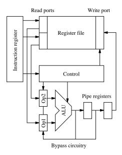
Fig. 11. Pipeline circuit block diagram
