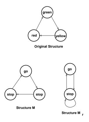
Fig. 5. Traffic light controller example
