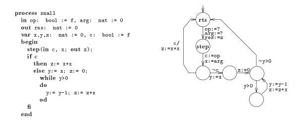
Figure 1: Example program and its flowchart
